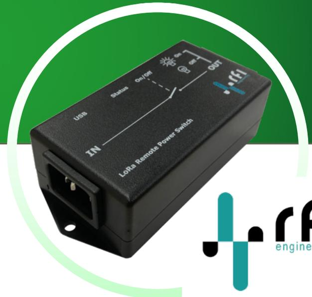
The LoRa Remote Power Switch is a smart LoRaWAN™ device for remotely controlling industrial and home appliances. The LoRa Remote Power Switch supports universal IEC320-C14 type input and IEC320-C13 output connectors to easily fit between the power cord and the device under control.
